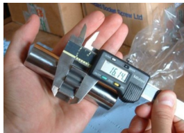
Photo 1 – shows gear width 1.614cm
